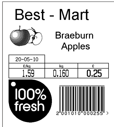
Figure 4-1 Current label using an EAN/UPC symbol with a Prefix 02 / 20-29
