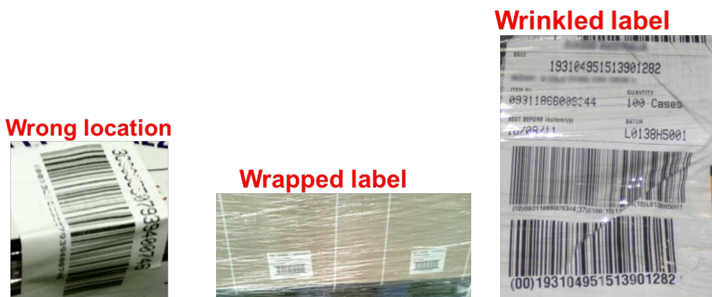
Figure 9-3 Examples of placement issues
